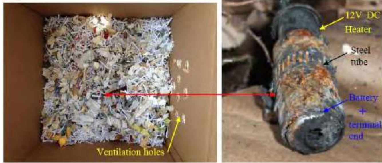
a) Fire-Starter in ventilated box with shredded paper, b) Post-fire condition.
